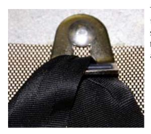
To attach the screen just slide the clip over the carriage bolt, and sung down the strap. If your system has the bolts screwed flush with the surface, unscrew the bolt about 1/8" then slide the clips on.
